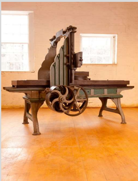
Lamson Goodnow & Co made metal planers and turret lathes then sold to the major armorers outfitting the Union, from the exhibition Shaping America at the American Precision Museum, Windsor, Vermont. www.americanprecision.org
